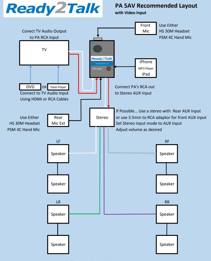
**Note:** If using 4 Ohm speakers connect pairs in SERIES
